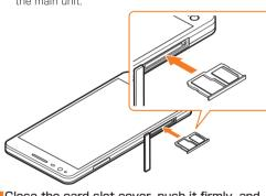
5 Close the card slot cover, push it firmly, and make sure that there is no gap between the cover and the main unit.
