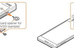
Put the au Nano IC Card 04 into the tray with the IC (metal) part downwards, insert the tray into the main unit, and then push it all the way straight into the slot.
