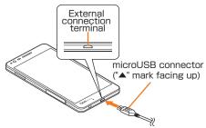
2 Insert the power plug of the common AC adapter 05 (sold separately) into a 100 V AC
