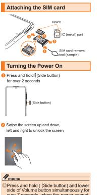
side of Volume button simultaneously for over 7 seconds, when the power cannot be turned off in the usual way or the screen freezes
